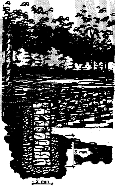
DRY OR MORTARED STONE WALL
